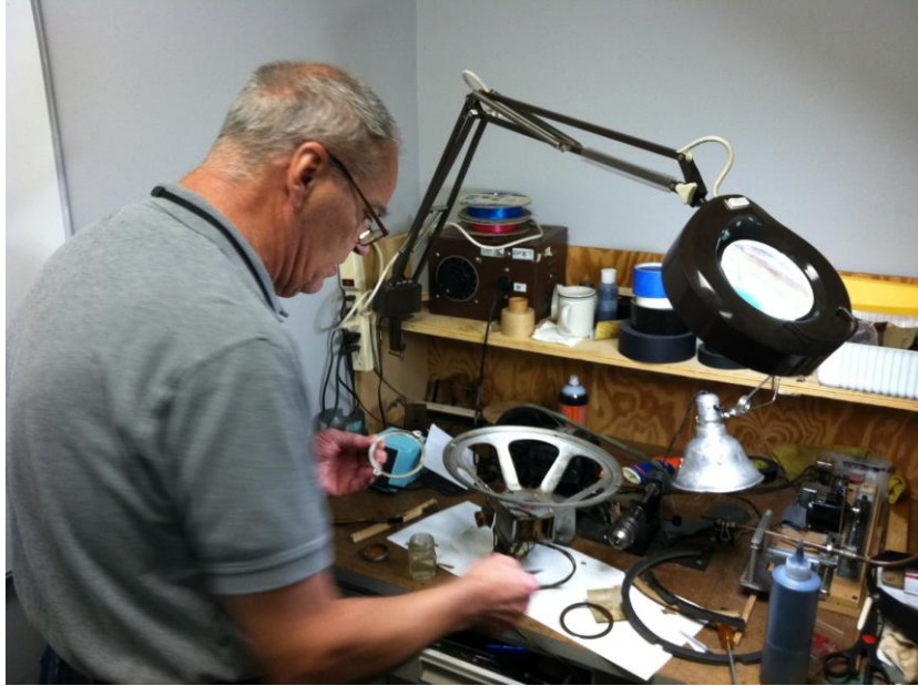
Dee Haynes repairing a customer speaker by replacing the cone and rewinding the voice coil
