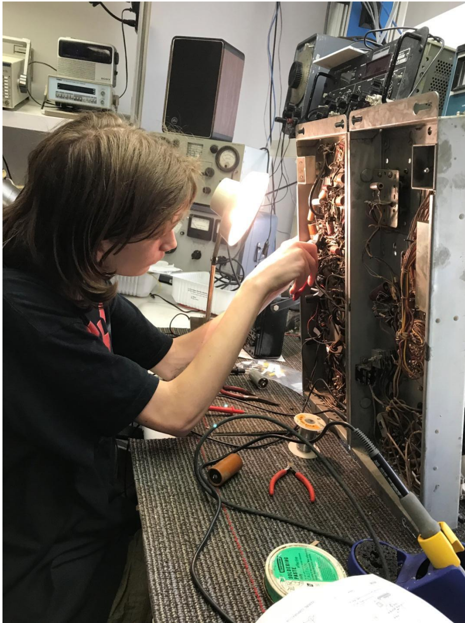
Student member Leo Barnhart working on the power supply of his jukebox amplifier.
