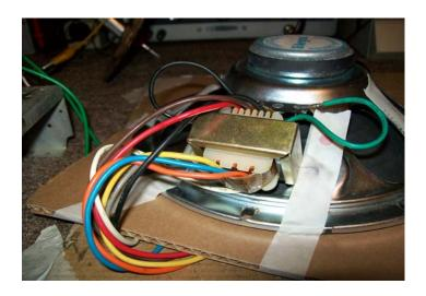
First I need to know the output impedance of a 6V6 tube. After doing a little research (RCA Tube Manual) I determined that the 6V6 when used as a Single Ended output tube was about 5,000 ohms impedance. Now all I need to know is which wires to use on the input of the audio transformer to match the 5,000 ohms to the 8 ohms on the speaker side of the transformer.
