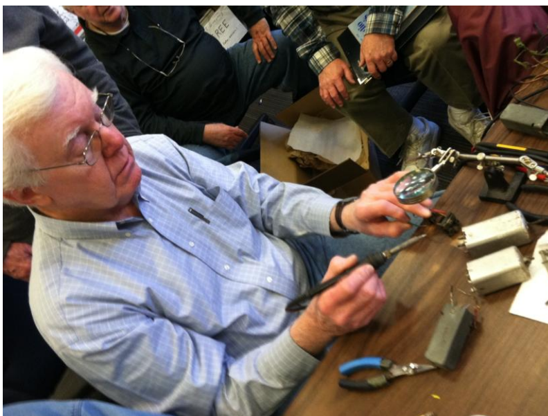
Mike Lord soldering the small wires on the IF coil
