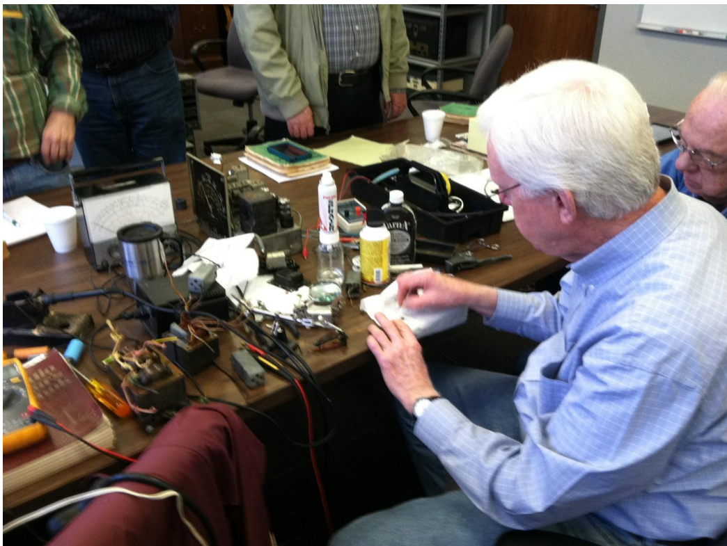
Mike Lord cleaning the mica washer on the IF tuning condenser
