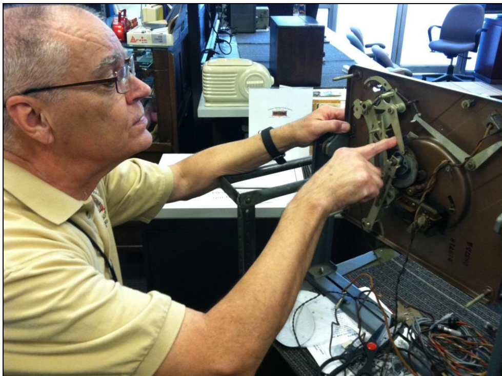
Dee Haynes working on a 1940's turntable using the turntable support device which allows the turntable to be rotated for ease of service. At the July Monday night meeting, Dee demonstrated how to "flock" the turntable platter on this turntable he is working on.
