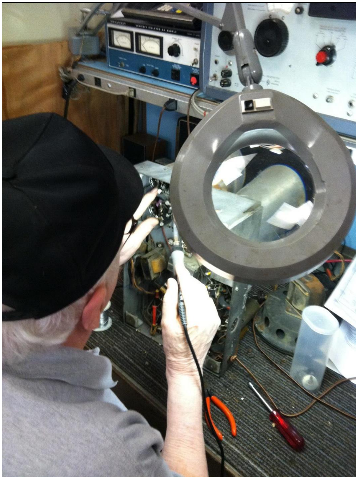
Jim Rogers replacing an IF coil, that was rewound by Dee Hayne, on a Philco 90
