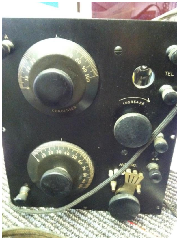
Maurice Lovelady brings in some unusual radios for repair and this one caught my eye. It is a 1922 Model HR Clapp-Eastham one tube radio.
