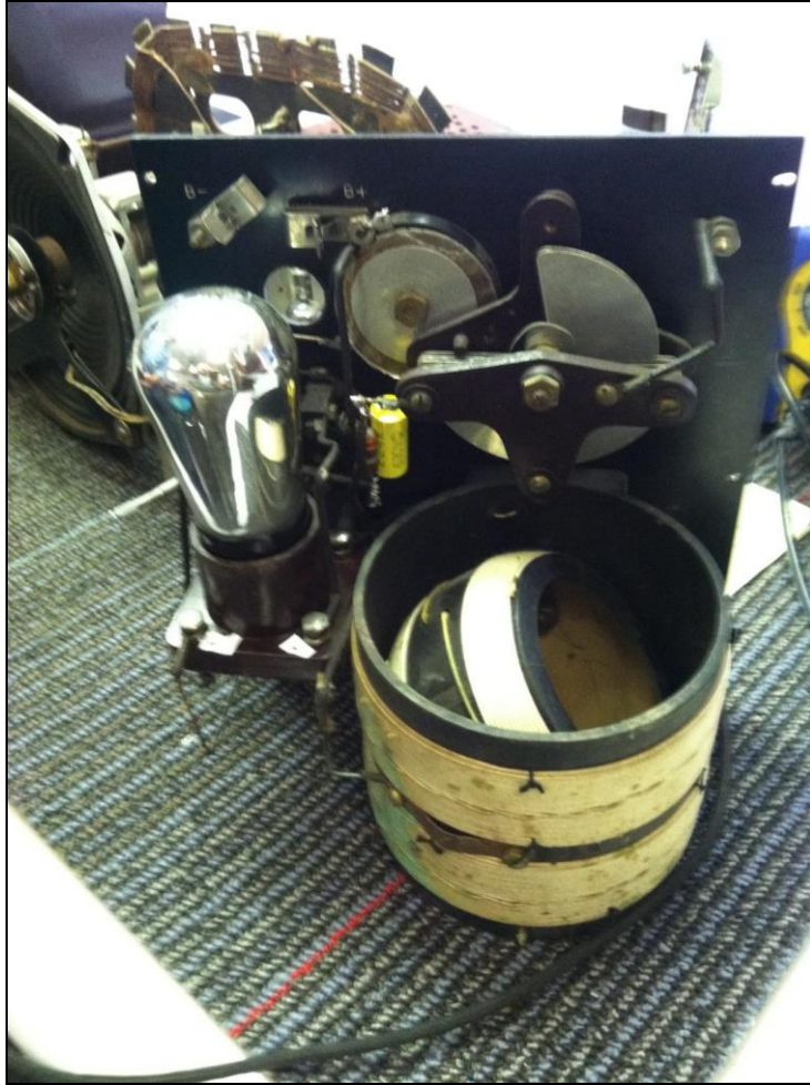
This is the inside of Maurice's Clapp-Eastham Radio showing the one tube circuit.
