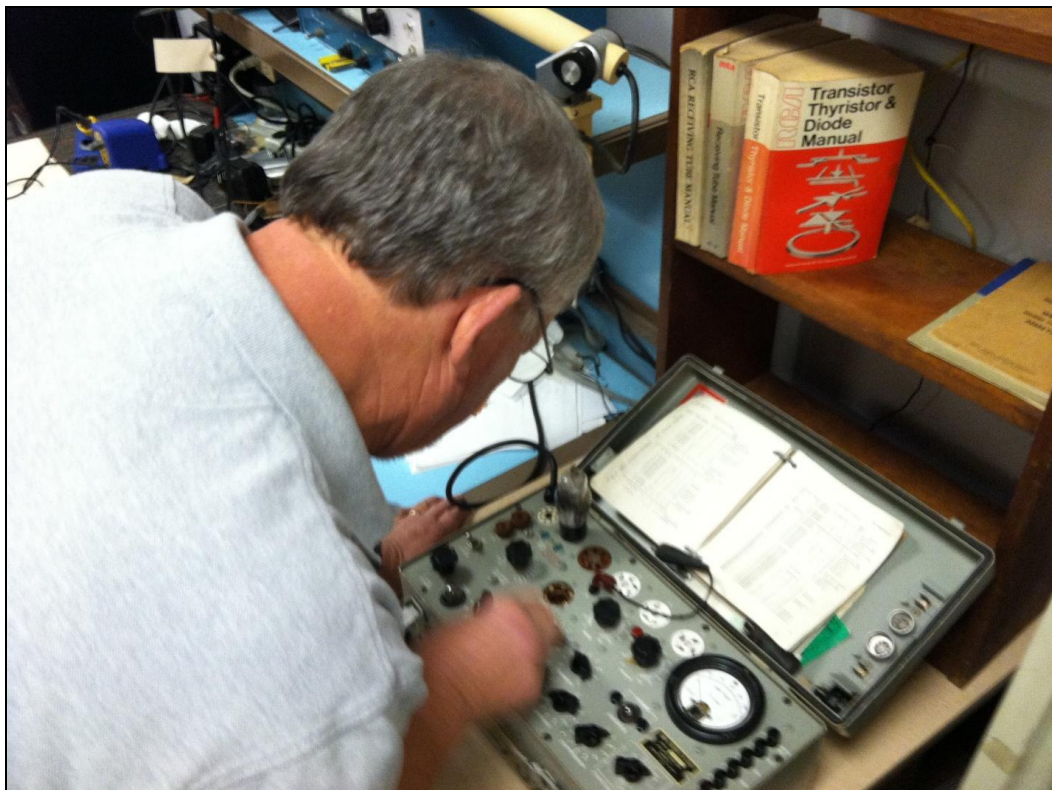
Doc Holladay using a military tube tester to check tubes in a radio he is restoring.
