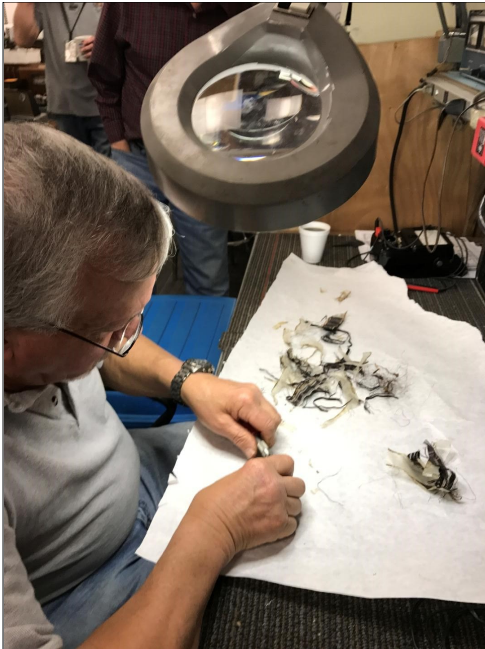
Doc Holiday unwinding a transformer to reclaim the form to wind a new transformer.
