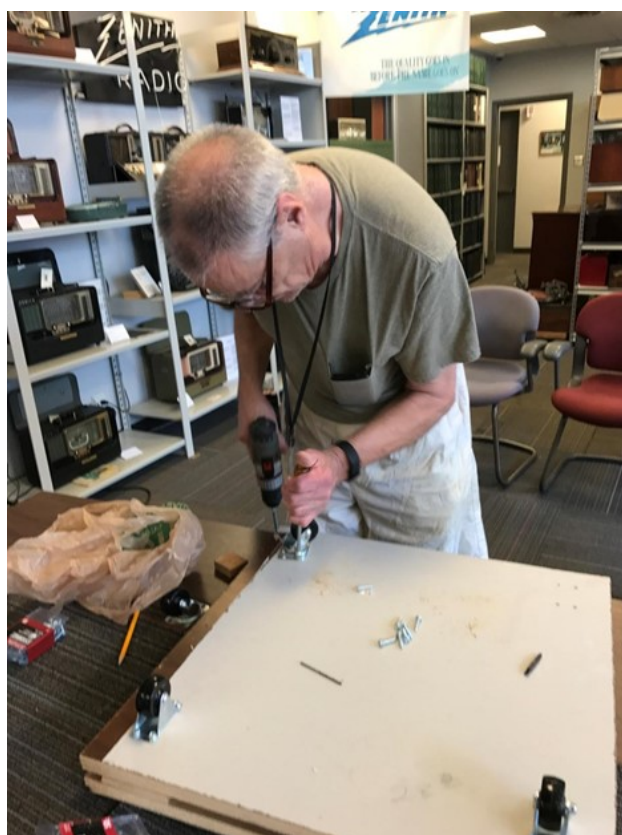
Dee Haynes installs the rollers on one of the rolling bases to be installed on the two transcription turntables, the studio mixer and the Ampex reel to reel tape recorder in the Rumore studio.
