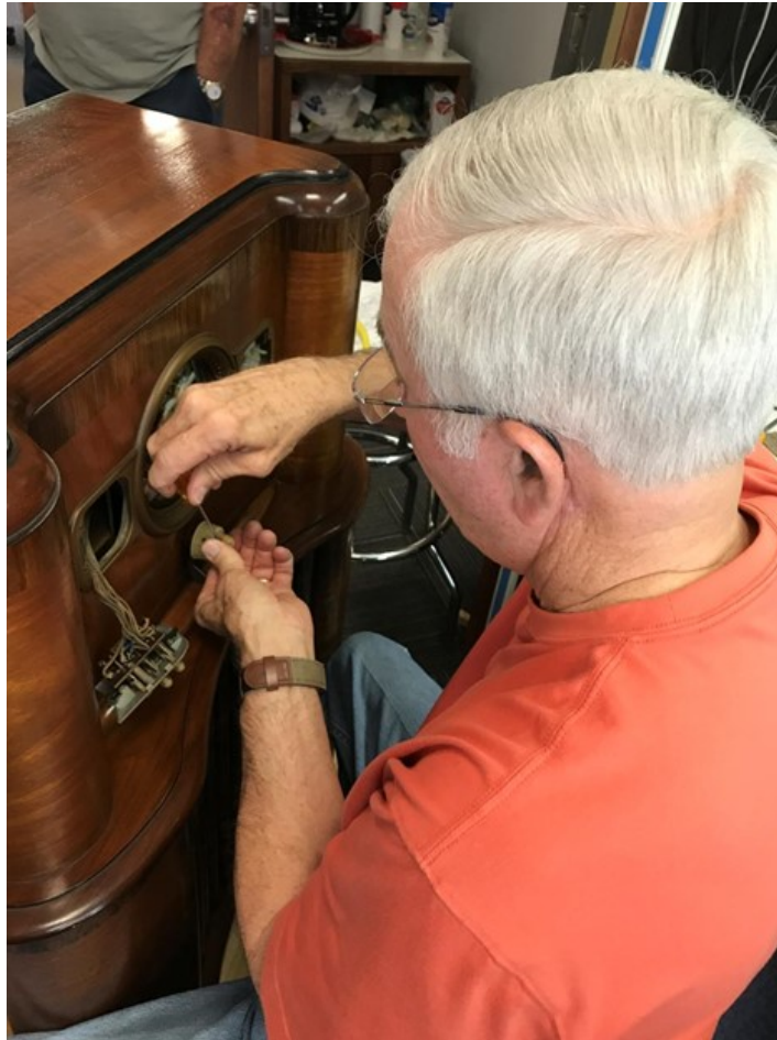
Frank Parker attaching the tuning knob as he completes this client restoration.
