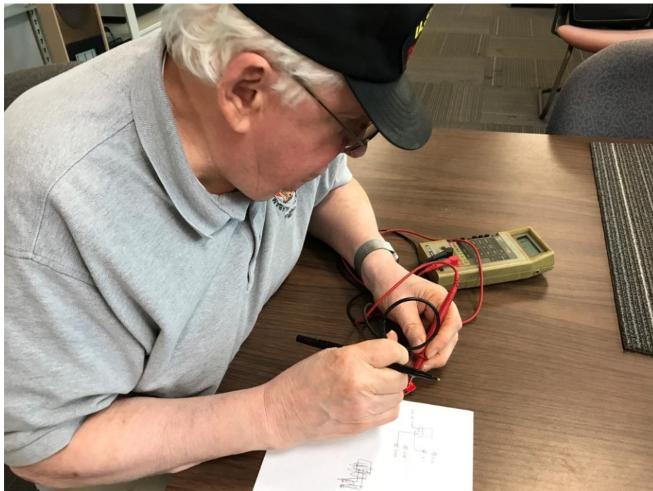
Jim Rogers using a digital volt-ohm meter to check a capacitor.
