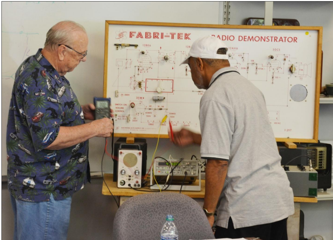
Joe Minor showing student Ron Hall how to check for continuity on a tube filament circuit.
