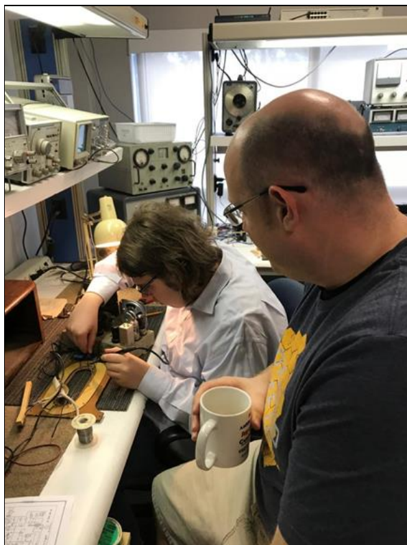
Milo Jones soldering the antenna leads on Josh White's (looking on) 1939 Packard Bell Model 5AC radio.
