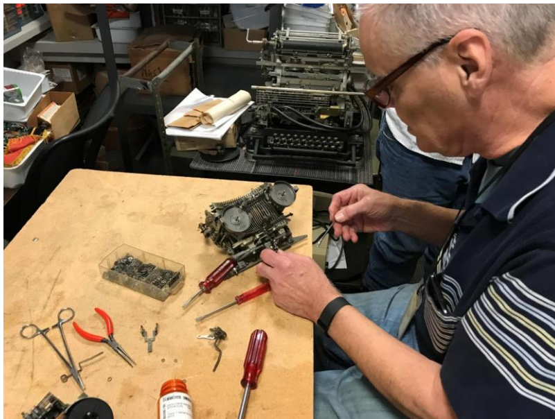
Dee Haynes replacing parts in a teletype drive unit at the Shop.
