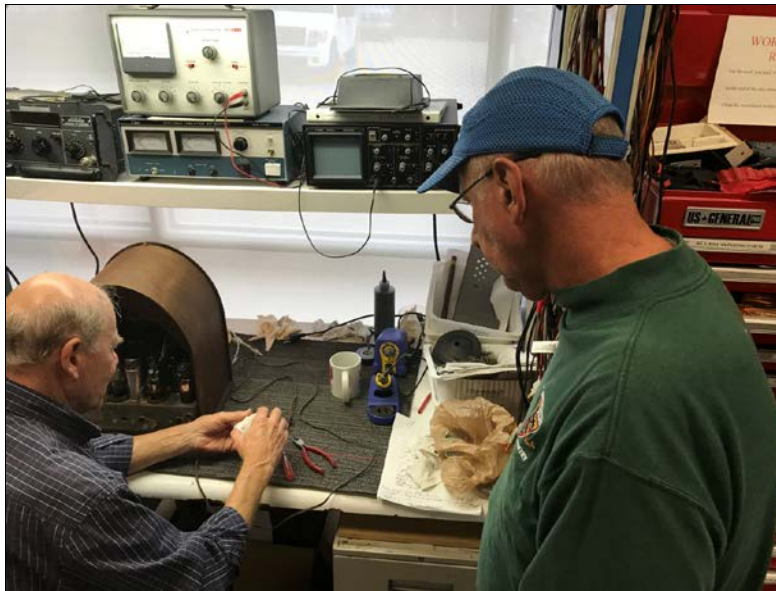
Don Letchman adding a cord switch to the Philco Cathedral Radio as Ray Giles looks on.
