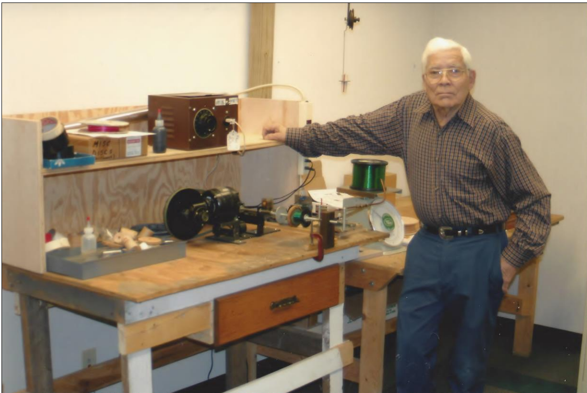
Marvin modified this coil winding machine to meet his production requirements.
