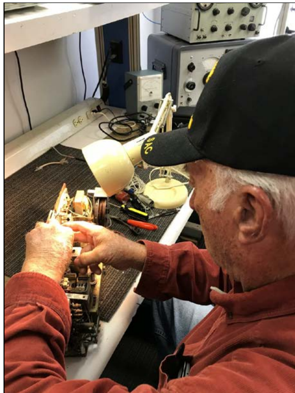
Maurice Lovelady replacing a tube he has just tested in a Zenith T.O. chassis
