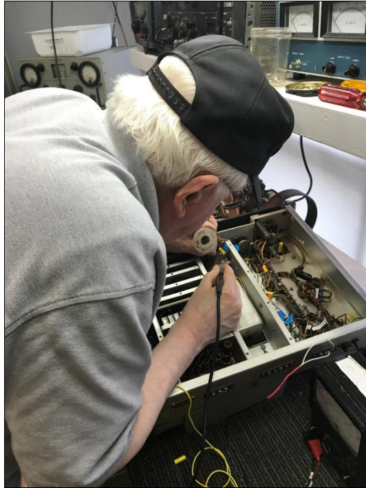
Jim Rogers soldering in a new capacitor in a donated Collins Model 75A1 circa. 1949 shortwave receiver
