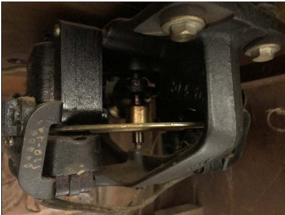
Victor Radio phono drive motor. It appears to have a speed governor system on the back side.
