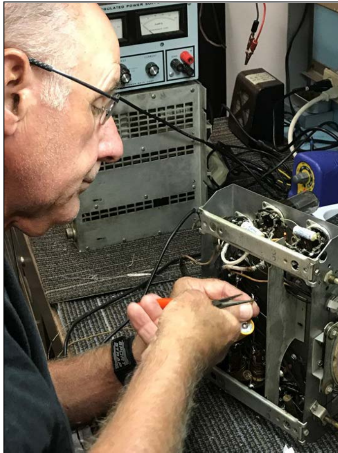
Ray Giles installing new power supply capacitors in a Crosley he picked up at one of our auctions.
