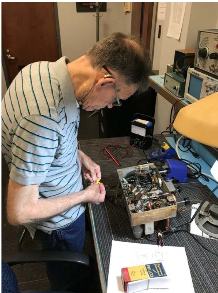
Jimmy Roberts replacing capacitors in the radio he is restoring.
